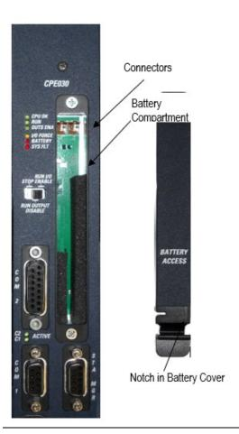
**Note:** An earlier version RX7i CPU may not have a slot in its battery door. For these CPUs, replace the door (supplied with the IC698ACC701 replacement battery).
