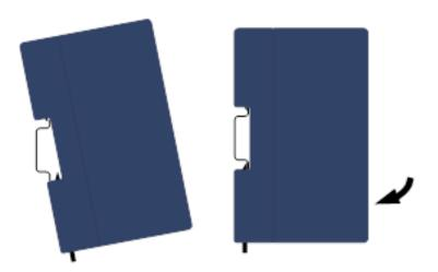
**Note:** To remove the Energy Pack from the DIN rail, use a small flat-blade screwdriver to pull down on the tab on the bottom of the Energy Pack and then lift the module off the DIN rail.
