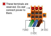
2. Insert the plug into the Input Power connector of the Energy Pack and securely tighten the attaching screws.
