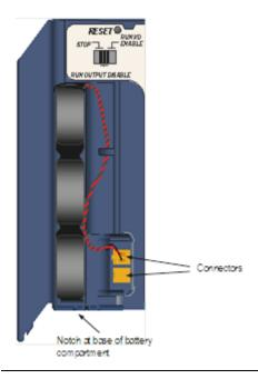
Figure 6: RX7i Battery Installation
