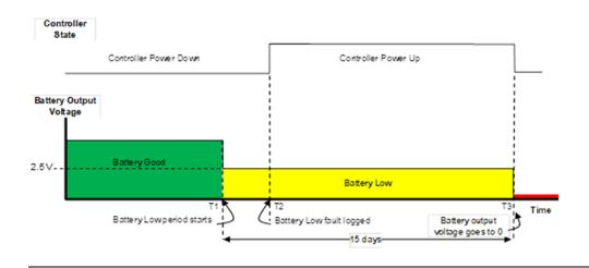
**Figure 1: Low Battery Countdown Example**
